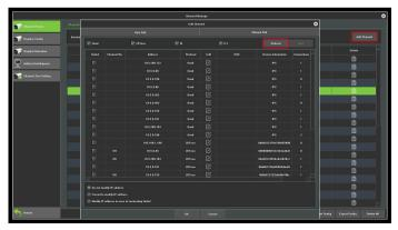
4. Select the checkbox for the device you want to add and edit the parameters in the corresponding text field, then click on [**OK**] to add it to the connection list.
