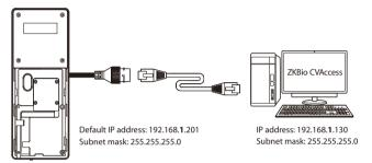
Tap on :: to enter the main menu. And then click on [Comm.] > [Ethernet] > [IP Address] to input the IP address.
